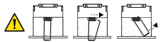
Ensure the two side springs are repositioned so they sit on the rim of the unit and are not an obstuction when fitting the sensor into the mounting box.
