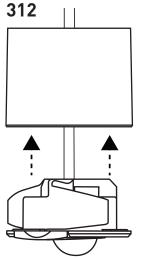
Note: Take care when placing the sensor into the mounting box. Ensure the fully fitted sensor sits secure and flush to the mounting box edge and no gaps are present.
